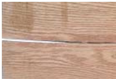
SPLIT: A lengthwise separation of the wood created as the wood dries. Shake is a separation between the annual growth rings.
