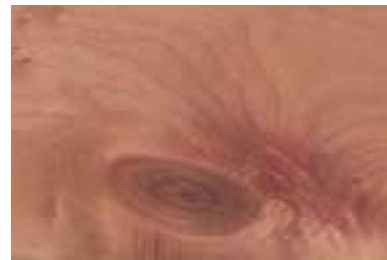
SOUND KNOT: A knot solid across its face, which shows no indication of decay.
